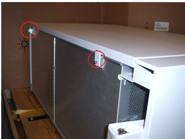
Figure 4 Remove shipping screws from back of top panel. The screws to remove are circled in this picture.
